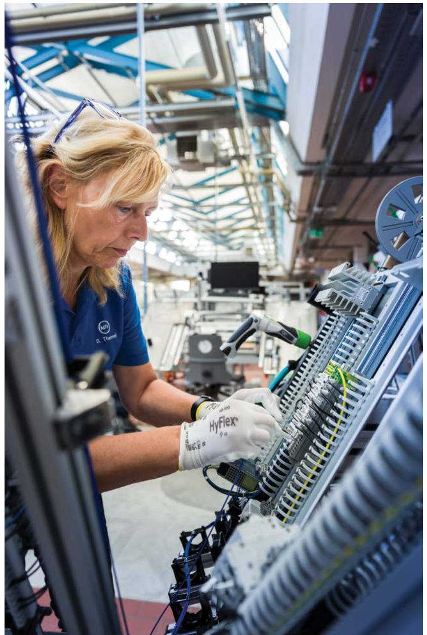
Ready to go: Precise and fast wiring of all components is already completed at Reinhausen. This saves customers valuable time.
